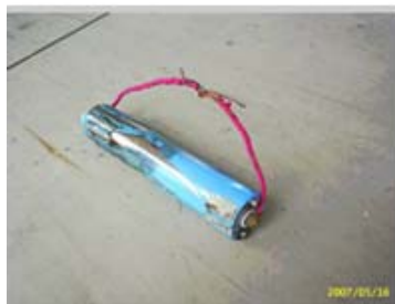
Short Circuit Test
